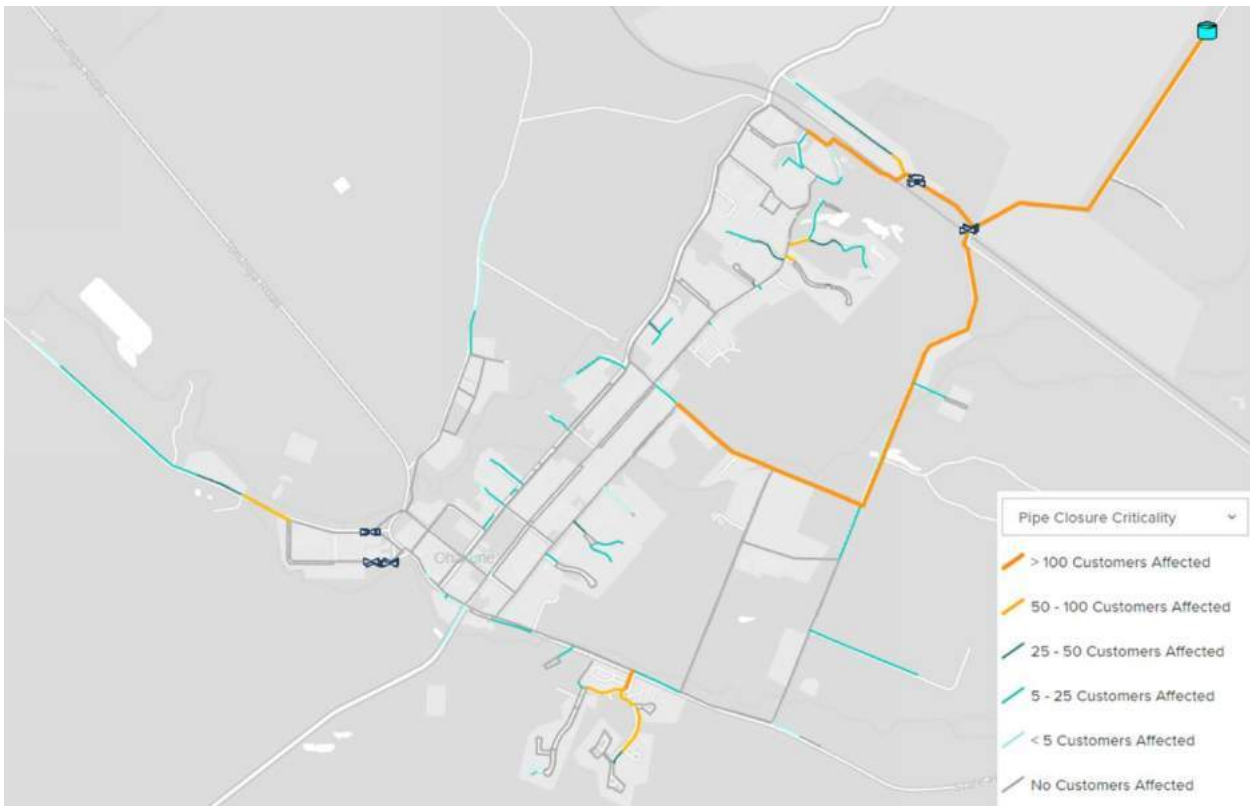
Figure 5.10: Pipe Criticality – 2031 Peak Day
