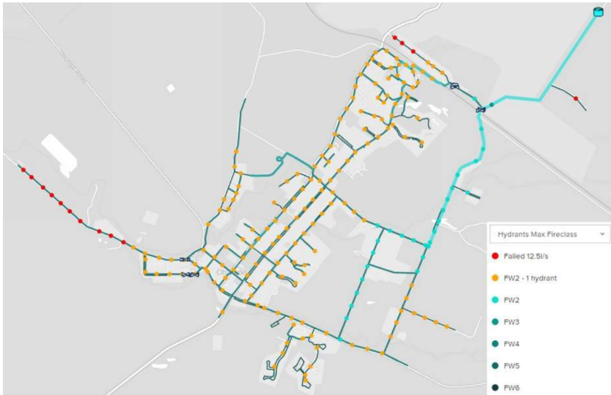
Figure 5.9: Hydrant Maximum Fire Class – 2031 Peak Day
